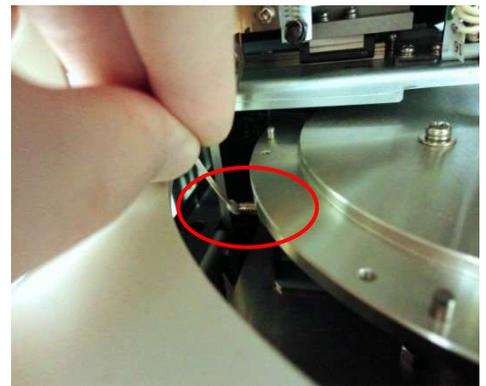
**7) Fix the removed cell holder with mounting screws.**
